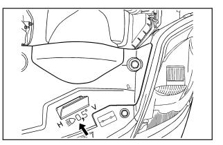
Locate the vertical headlamp aiming screws. They are located under the hood near each headlamp assembly. First lift the flap to access either of them. Each one is the top outboard screw by the "V" on the cover panel next to the aiming flap.
